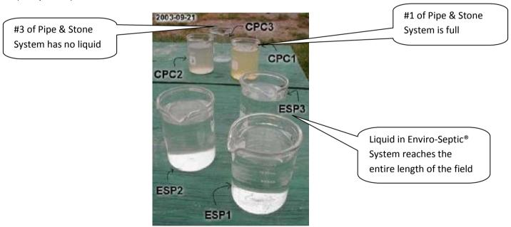
Compare that with the three samples taken along the Enviro-Septic® row, which shows leachate reaching the far end of the field as seen by the liquid collected by the third beaker. Clearly, the BTL is providing even distribution, which is a vital service in the proper, long-term life of the system.
