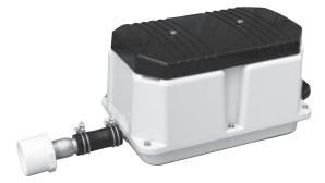
B. If using the linear blower (Thomas model LW250) attach the 1-inch galvanized male adapter to the blower using the supplied hose and clamps. Next attach the 2-inch Schedule 40 PVC reducer to the male adapter, then connect the PVC line to the reducer using PVC solvent.
