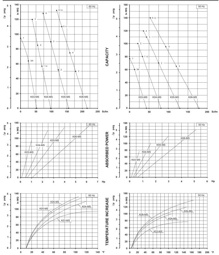
Curves refer to air at 68°F temperature and 29.92 In Hg atmospheric pressure (abs) measured at inlet port. Values for flow, power consumption and temperature rise: +/-10% tolerance. Data subject to change without notice.
