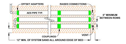
It is acceptable to substitute Advanced Enviro-Septic<sup> $\mathbb{M}$ </sup> for Enviro-Septic<sup> $\mathbb{M}$ </sup> provided all of the conditions (1 – 4) above are met and amendments are submitted to NH DES prior to a request for inspection.
