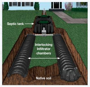
Effluent flows into the Infiltrator Quick4 leachfield where it is naturally purified as it percolates down through the soil.
