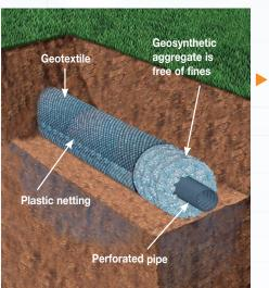
EZflow geosynthetic systems replace stone in a traditional system reducing compaction and fines.
