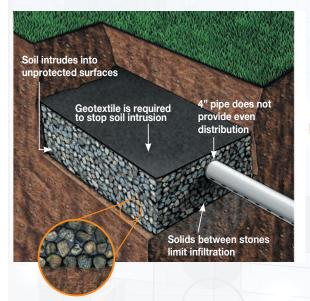
Stone and pipe systems can fail because solid matter clogs the space between the stones.
