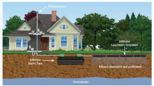
A standard septic system has two components: a septic tank and a leachfield.
