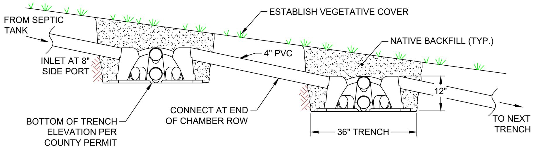
\*NUMBER OF ROWS DETERMINED BY DESIGN AND CENTER TO CENTER SPACING PER CODE.
