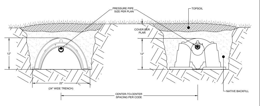
TRENCH LENGTH, NUMBER OF CHAMBER AND INSTALLATION DEPTH PIPE SIZE, ORIFICE SIZE AND SPACING, DETERMINED BY DESIGN
