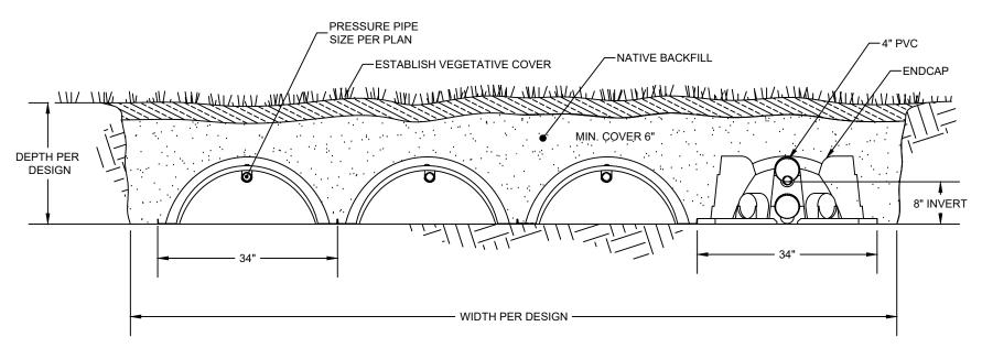
LENGTH, NUMBER OF CHAMBERS AND INSTALLATION DEPTH DETERMINED BY DESIGN
