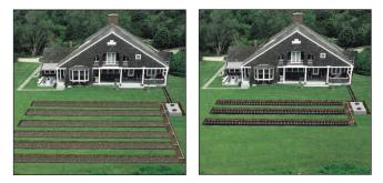
Traditional full-size stone and pipe leachfield vs. reduced size chamber system leachfield.
