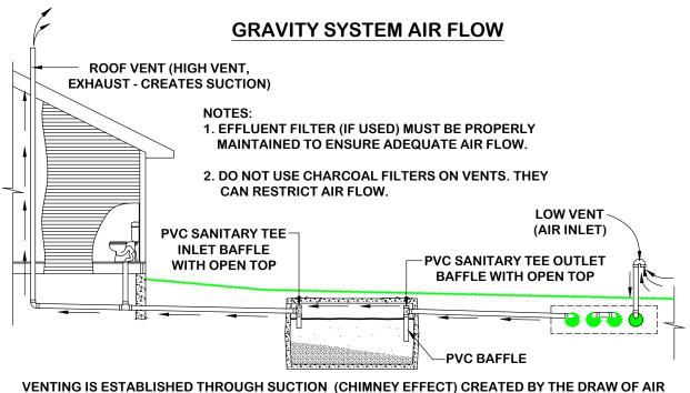
FROM THE HIGH VENT, WHICH DRAWS AIR INTO THE LOW VENT AT THE LEACH FIELD THEN THROUGH THE SEPTIC TANK AND EXHAUSTED THROUGH THE (HIGH) ROOF VENT.
