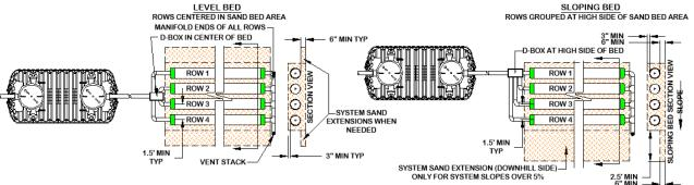
PEI and DEQ do not require installation of pipe rows in a straight line. In fact, it is always preferable to follow the contour of the land. Never install the leachfield in floodways, at the base of slopes, or in depressions where runoff water could flood the leachfield. Construct leachfields in areas with good surface drainage, where the water cannot pond over the leachfield.
