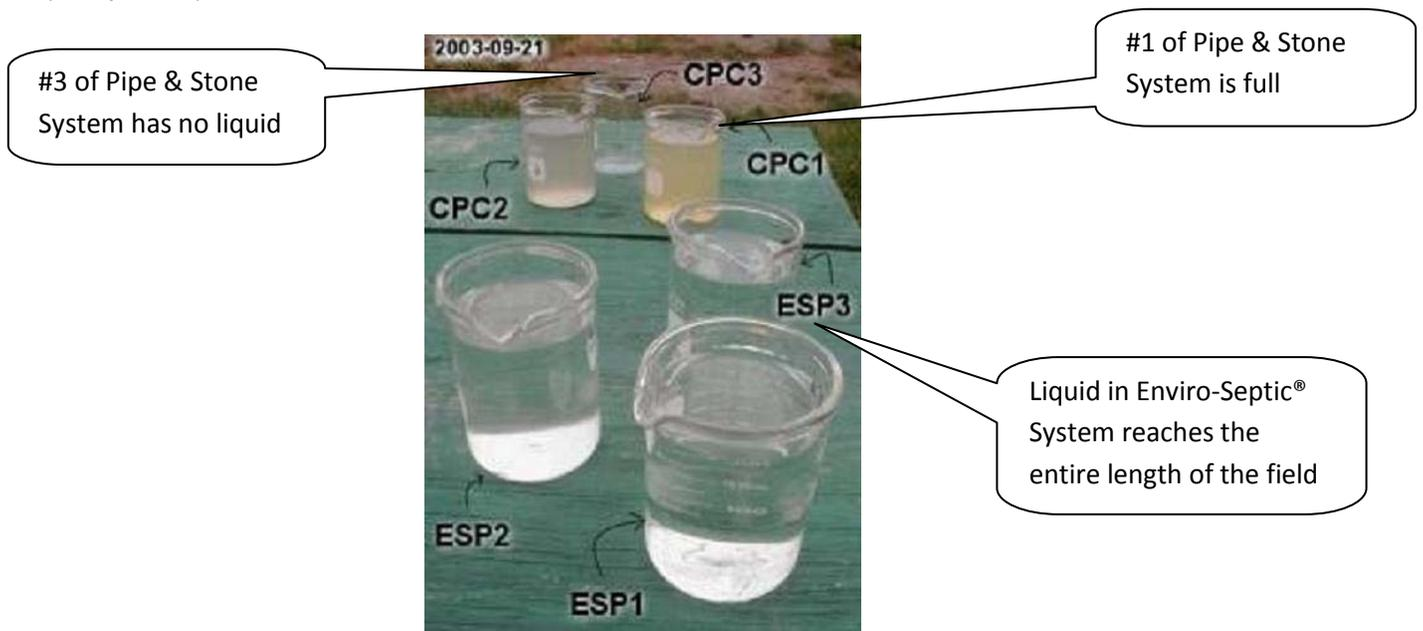
Compare that with the three samples taken along the Enviro-Septic<sup>®</sup> row, which shows leachate reaching the far end of the field as seen by the liquid collected by the third beaker. Clearly, the BTL is providing even distribution, which is a vital service in the proper, long-term life of the system.
