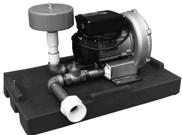
A. If using the regenerative blower (FPZ model SCL06) attach the 1x6 galvanized nipple to the 1-inch galvanized elbow, then attach the 2-inch Schedule 40 PVC reducer to the 1-inch galvanized nipple. Next connect the PVC line to the PVC reducer using PVC solvent.
