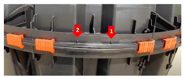
The deformations are located at the outlet end of the tank between the upper and lower serial numbers. Attaching the two mid-seam clips in this area can be difficult. The mid-seam curls up and away from the centerline and is thicker in the deformed area. All but the two clip bosses identified in the photo above should receive clips with relative ease. These two deformed clip bosses will receive clips if installed in a specific direction and specific order.
