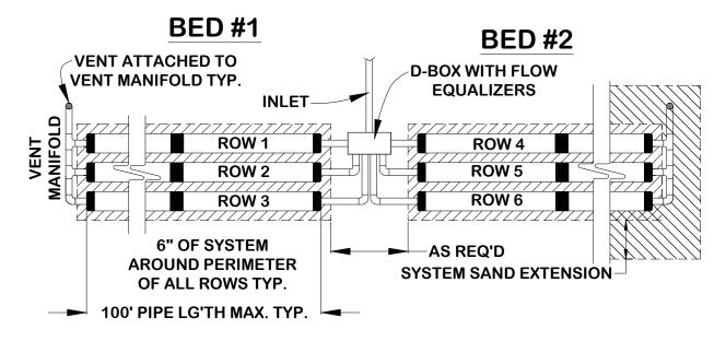
**Note**: This Multiple Bed configuration may be used in all soil types. See previous page for minimum bed separation distances.
