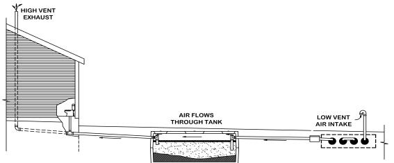
Air flow is established by the High Vent's chimney effect, which draws air into the Low Vent, through the Advanced Enviro-Septic® pipes, through the septic tank and exhausting through the roof vent.
