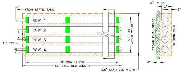
Alternate bed configurations for Example #1: (2 rows of pipe 100 ft long) or (5 rows of pipe 40 ft long). Note: for complete description of Basic Serial Distribution (see sect. 9.0, p 10).
