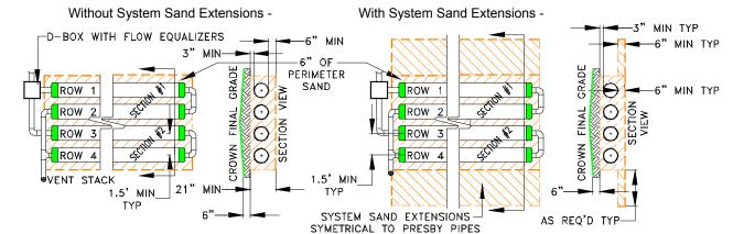
g) When the vent manifold is on the same side as the serial section inlets, the manifold runs over the top of these inlets.
