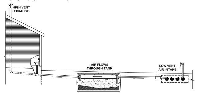
Air flow is established by the High Vent's chimney effect, which draws air into the Low Vent, through the Advanced Enviro-Septic® pipes, through the septic tank and exhausting through the roof vent.
