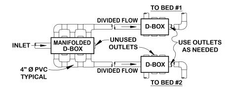
**Note**: Utilizing every other outlet will provide room for required piping and allow for easier installation. Install flow equalizers on all used outlets.
