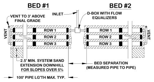
**Note**: This Multiple Bed Basic Serial distribution configuration may be used in all soil types. See previous page for Minimum Bed Separation distances.
