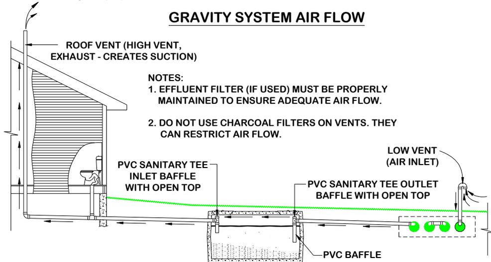
Venting is established through suction (chimney effect) created by the draw of air from the high vent, which pulls air from the low vent at the leachfield, through the septic tank, and exhausts it through the high (roof) vent.
