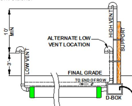
d) Illustration of gravity system air flow:
