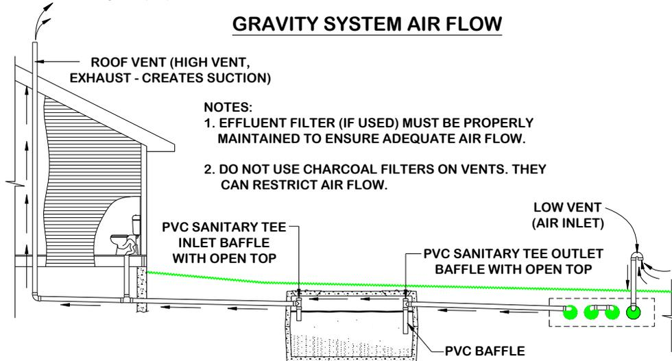
Venting is established through suction (chimney effect) created by the draw of air from the high vent, which pulls air from the low vent at the leachfield, through the septic tank, and exhausts it through the high (roof) vent.
