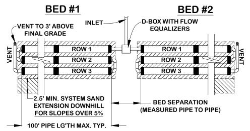
**Note**: This Multiple Bed Basic Serial distribution configuration may be used in all soil types. See previous page for Minimum Bed Separation distances.
