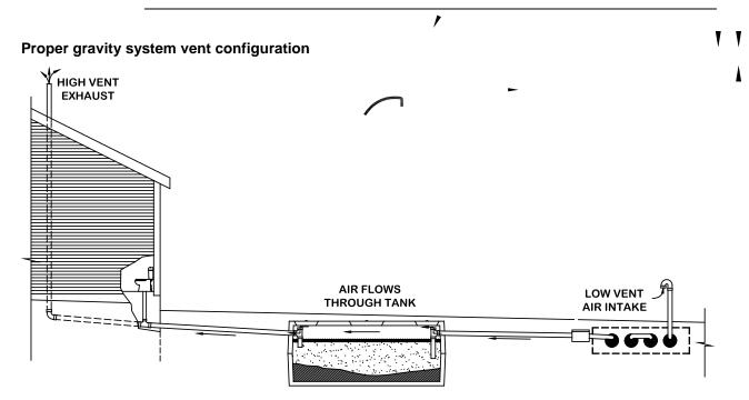
Air flow is established by the High Vent's chimney effect, which draws air into the Low Vent, through the Advanced Enviro-Septic® pipes, through the septic tank and exhausting through the roof vent.
