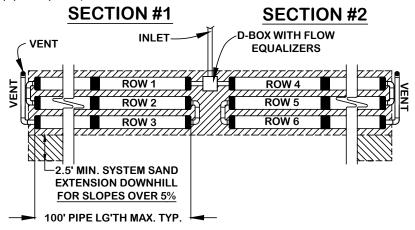
D-Box Distribution Configuration (a.k.a. "Parallel" or "Finger" configuration)
