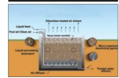
Wastewater treatment for small and remote applications requires simple and robust solutions. With this objective in mind, BIOSOR has been developed over 10 years of R&D by the Quebec government Centre de Recherche Industriel du Quebec (CRIQ). BIOSOR is low maintenance and requires no operation. Also, no biologic sludge needs to be managed. All it takes is a media change-out every three to five years.
